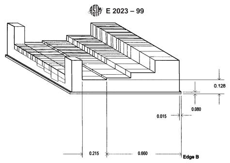
Unless otherwise specified, use the following: Dimensions are in inches. Tolerances on machined dimensions:  $XX = \pm .01$   $XXX = \pm .01$
