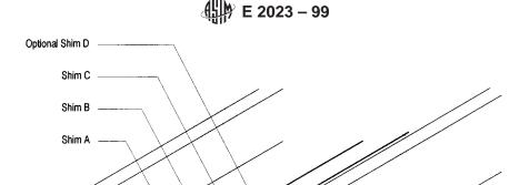
Note 1—See Fig. 4. FIG. 5 Shims in Channels
