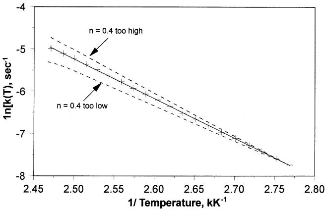
FIG. 2 Plot of In[k (T)] versus 1/T
