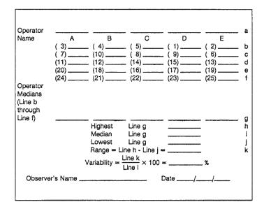
NOTE—(B) denotes test sequence. FIG. X1.1 Data and Calculation Sheet for Multiple-Operator **Reproducibility Test**
