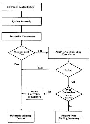
FIG. X3.1 Preseason Binding Inspection
