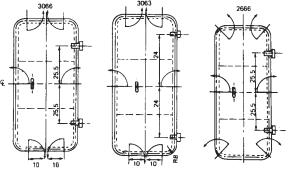
Remarks 1. Stiffeners shall be spaced to divide the doorway into three equal parts.
