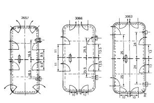
Remarks: 1. Stiffeners shall be spaced to divide the doorway into four equal parts.
