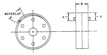
Note 1—Maximum overlap is 8 in. (203 mm). Note 2—Minimum overlap is 1 in. (25 mm). FIG. A1.1 Shield Length
