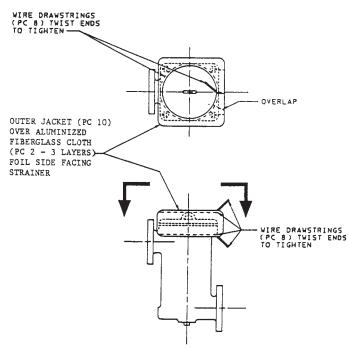
FIG. 4 Spray Shield for Simplex Strainer
