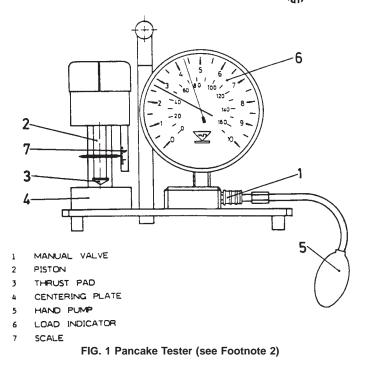
9.4 Mount thrust pad (Fig. 1, Item 3) by screwing it into the piston rod. Note that this step is only applicable if a special thrust pad is needed for the pancake to be tested. Normally, a standard thrust pad is part of the basic test apparatus.
