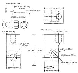
FIG. 1 Gripping Device for Shear Testing
