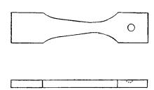
FIG. 9 Tapered Beam Configuration for Bend Testing
