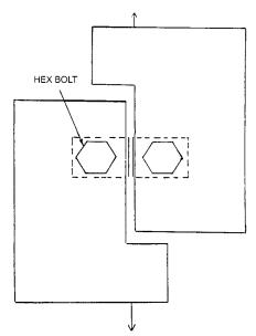
FIG. 4 Drawing of the Recommended Shear Test Specimen
