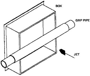
FIG. X2.1 Basic Layout of a Jet Fire Test
