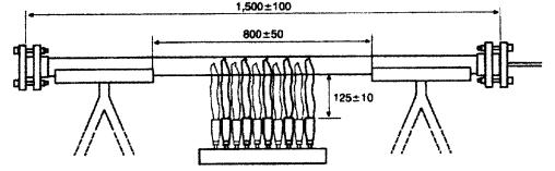
FIG. X2.2 Basic Layout of an Impinging Flame Test
