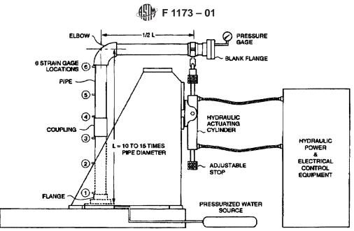
FIG. X4.1 Typical Low-Cycle Mechanical Fatigue Endurance Test Setup
