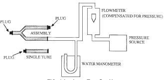
FIG. 1 Leakage Test Set-Up
