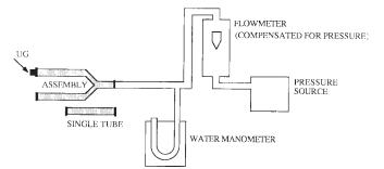
FIG. 3 Expiratory Pathway Resistance Test Set-Up
