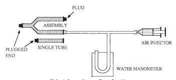
FIG. 4 Compliance Test Set-Up
