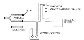
FIG. 2 Inspiratory Pathway Resistance Test Set-Up
