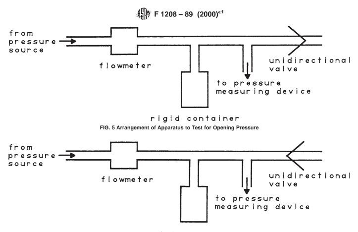
rigid container FIG. 6 Arrangement of Apparatus to Test for Reverse Flow
