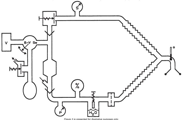
FIG. 3 Illustration of the Use of Graphic Notation (Symbols) in a Circle Absorber System
