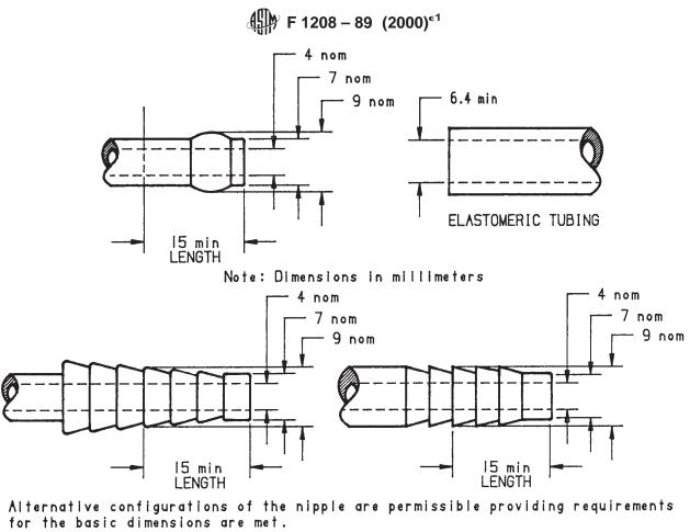
FIG. 7 Examples of Fresh Gas Inlet Nipples
