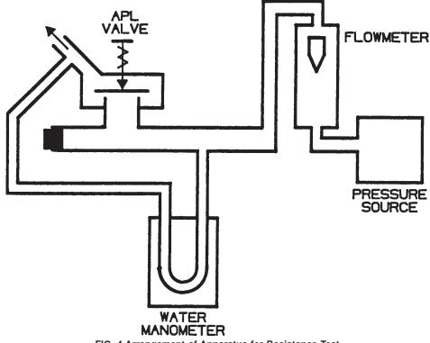
FIG. 4 Arrangement of Apparatus for Resistance Test
