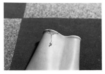
FIG. 25 Tracking—Insufficient Immersion Depth
