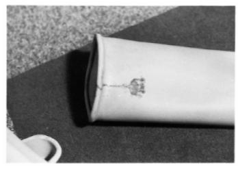
FIG. 26 Tracking—Contaminated Dielectric Fluid
