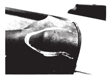
FIG. 19 Ozone Cracks
