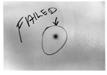
FIG. 4 Breakdown (Dielectric Failure)
