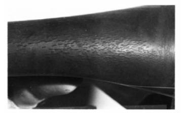
FIG. 18 Ozone Cracks
