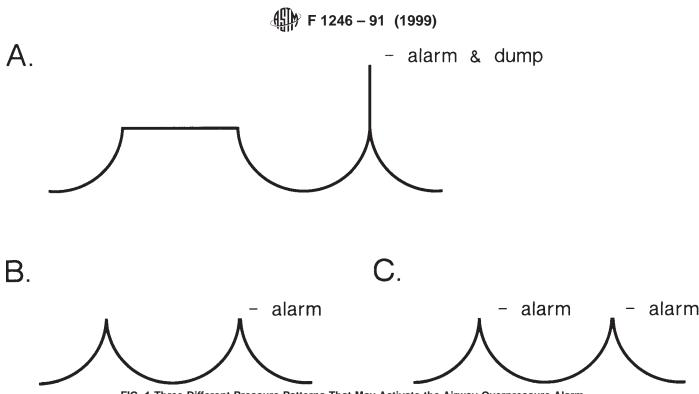
FIG. 1 Three Different Pressure Patterns That May Activate the Airway Overpressure Alarm
