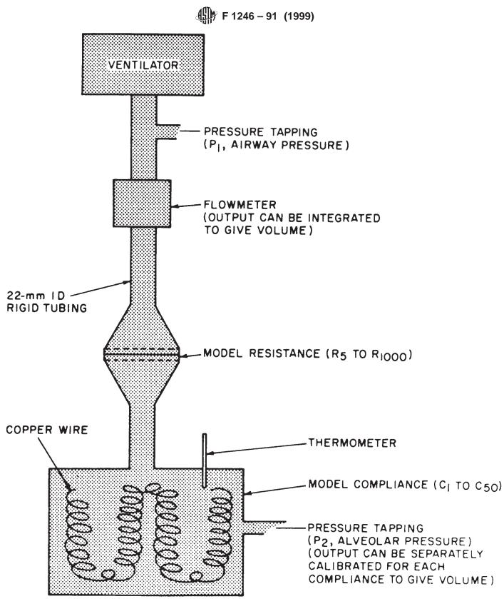
FIG. A1.1 Representative Passive Lung Model
