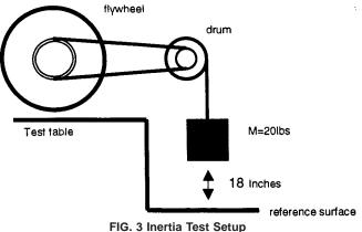
7.7.1.3 *Acceptance Criteria*—No permanent vertical displacement of the of the pedal shall have occurred.
