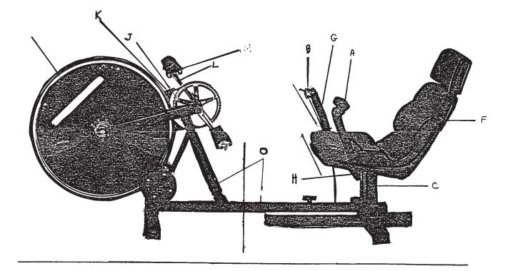
A - Load/Speed Indicator B - Load Adjustment
