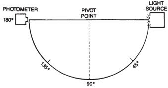
FIG. 4 Apparatus Set-Up for Source Measurement
