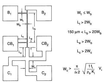
FIG. 1 Design Features for the Cross-Bridge Test Structure
