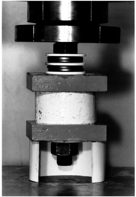
FIG. 2 Typical Arrangement to Apply the Compression Load and Hand Tighten the Nut
