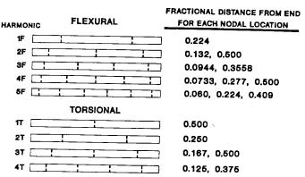
FIG. 5 Dynamic Modulus Resonant Modes and Nodal Locations
