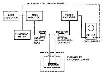
FIG. 1 Block Diagram of a Typical Test Apparatus
