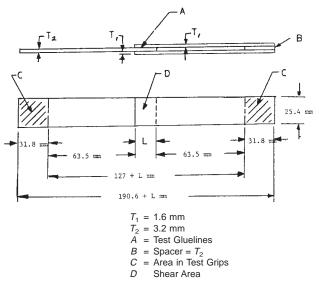
FIG. 1 Form and Dimensions of Type A Specimens
