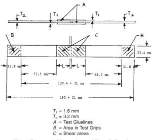
FIG. 2 Form and Dimensions of Type B Specimen
