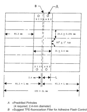
FIG. 4 Form and Dimensions of Standard Test Panel for Type B Specimens
